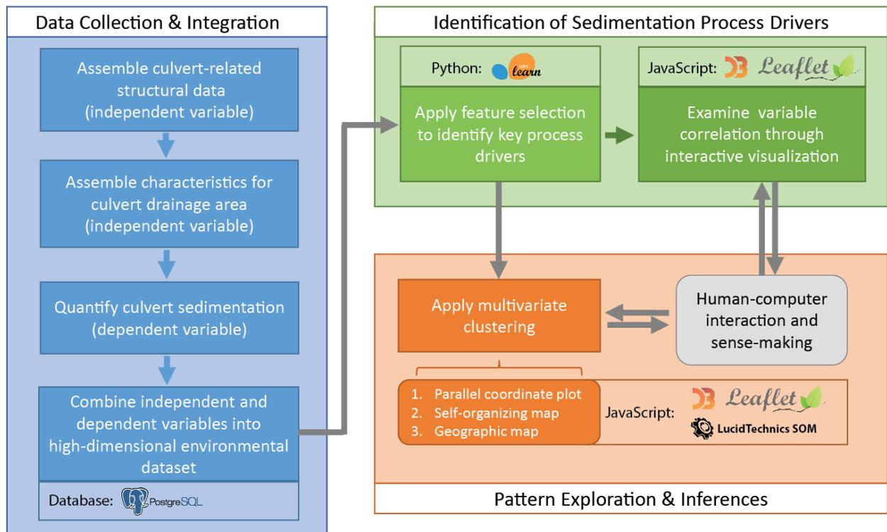
Fig. 1. The analytical pipeline of the platform.
