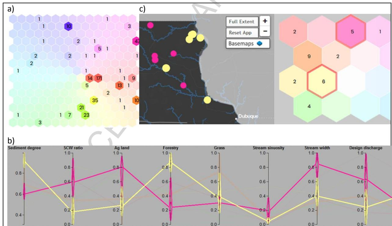
Fig. 5. The SOM visualizations: (a) hexagonal layout of SOM nodes, (b) edge-bundling PCP that displays the multivariate patterns and overall trends of each culvert clusters, and (c) spatial locations of culverts contained in individual cluster (node/hexagon).
