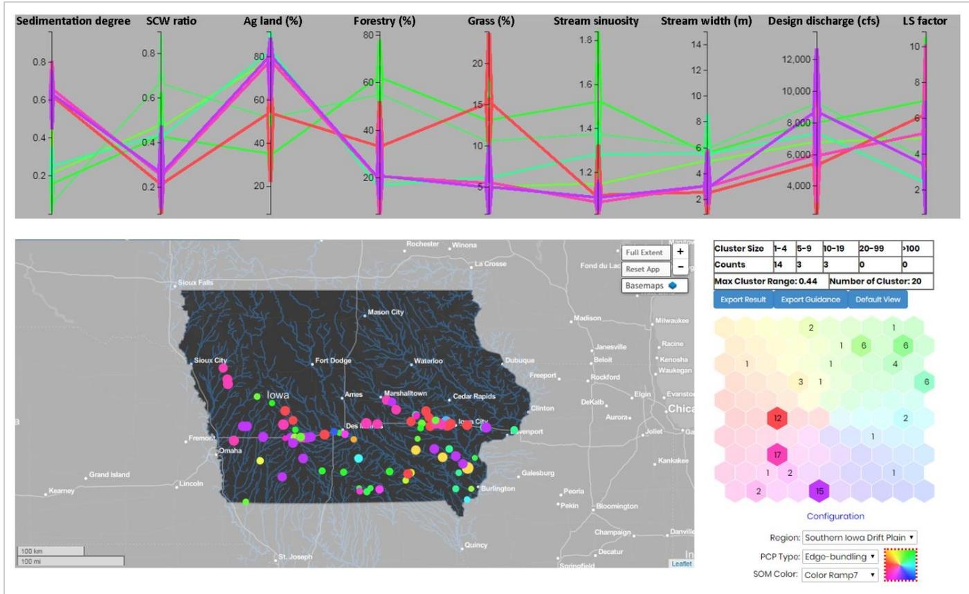
Fig. 8. Empirical relationships between drivers and the culvert sedimentation degrees in the Southern Iowa Drift Plain regions.
