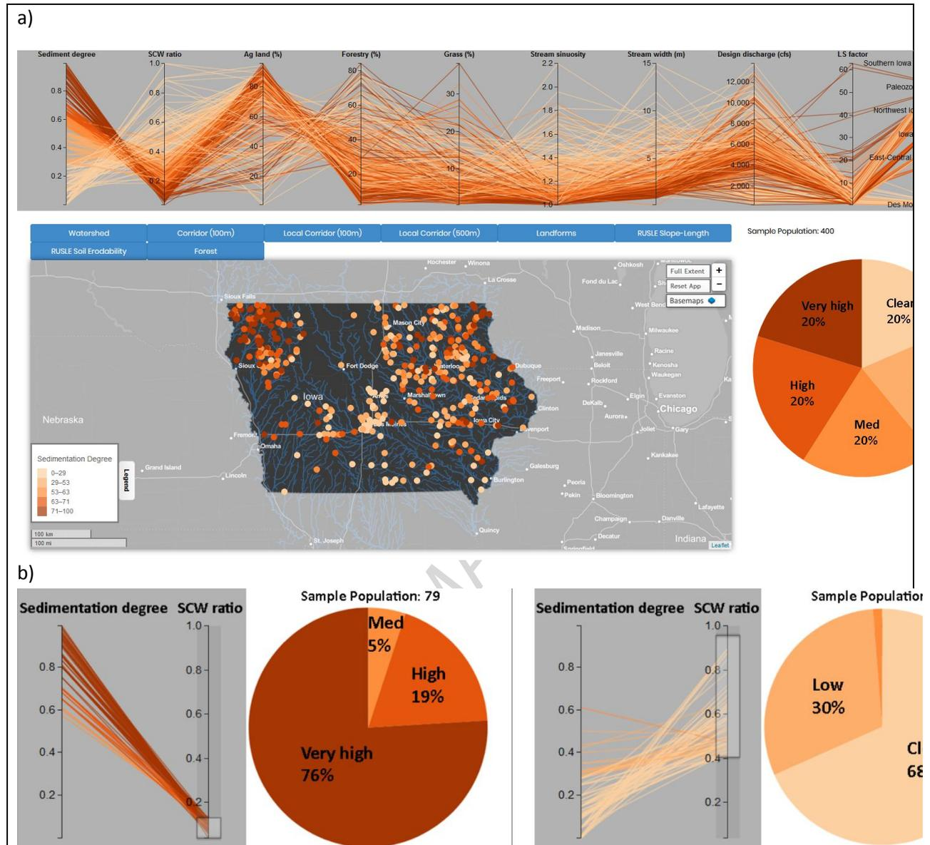
Fig. 4. Interfaces for (a) visualizing culvert sedimentation datasets in both the geographic space (web map) and the multi-dimensional attribute space (PCP and pie chart) and (b) examining the dependency between the sedimentation degree and SCW ratio.
